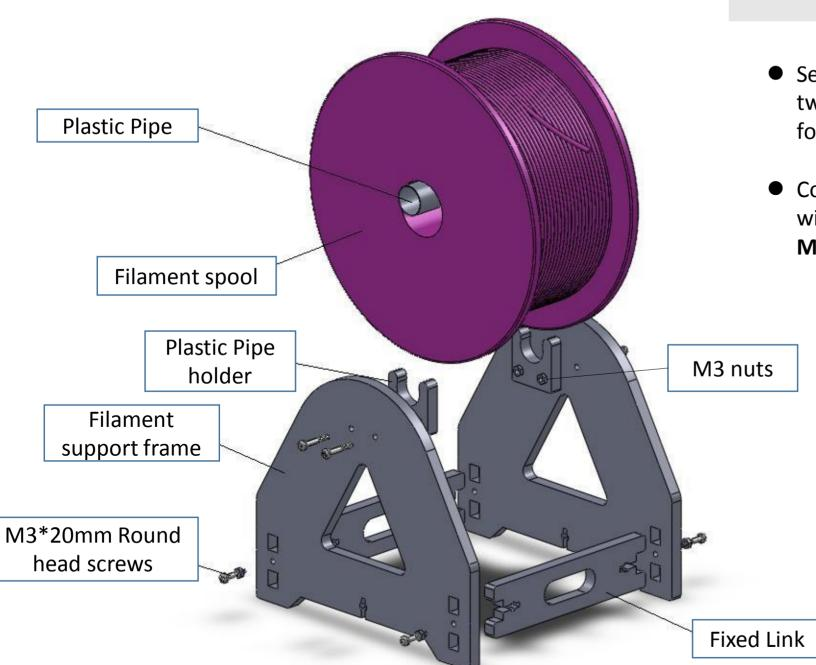
Separately put two Plastic Pipe holder on two Filament support frame, locking with four M3\*20mm Round head screws & nuts.
